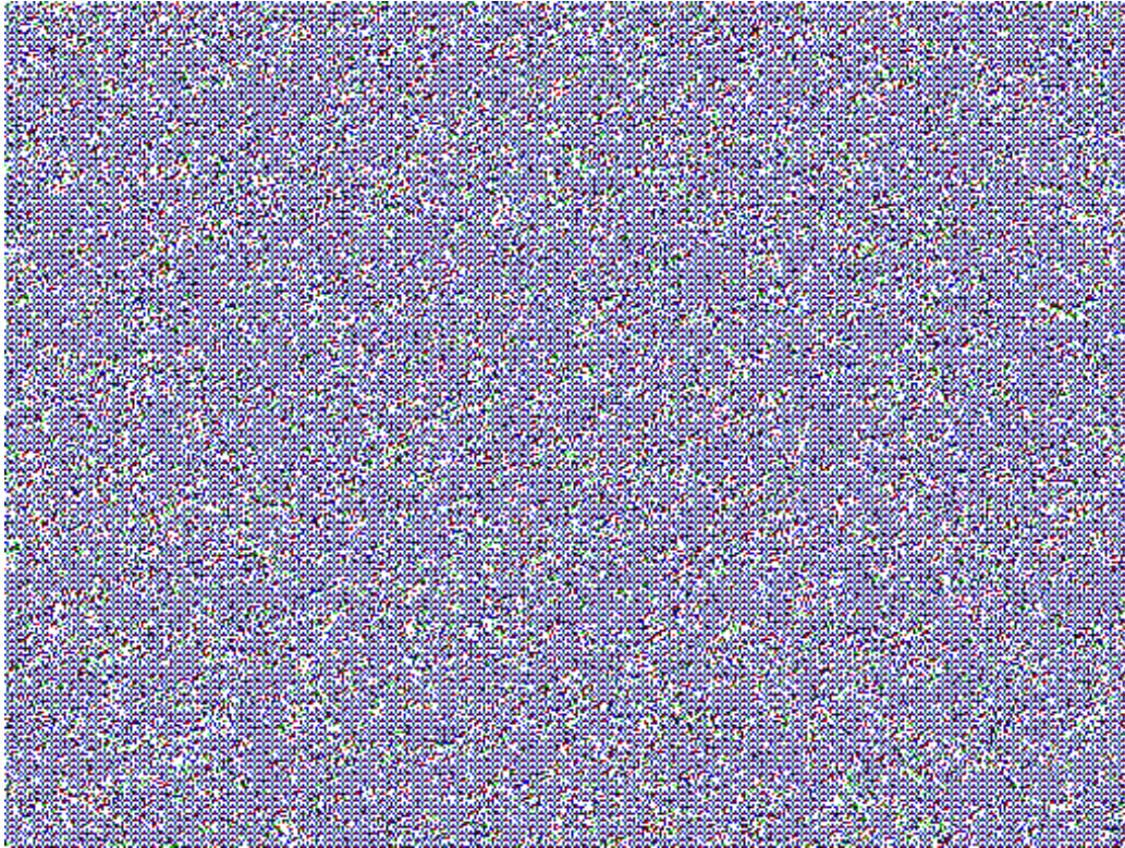
Fig. 8.2. OpenSSL AES timings for 128 keys and 128 inputs on a Pentium M. This picture is a 128 \times 128 array of blocks. There is one key for each row of blocks; there is one input for each column of blocks. The pattern of colors in a block reflects the distribution of timings for that (key, input) pair. There is tremendous variability among blocks in this picture. Reader beware: this picture is easily corrupted by low-resolution displays.
